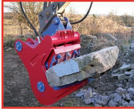
Breaking large slabs of demolition waste (No Breaker Required)
