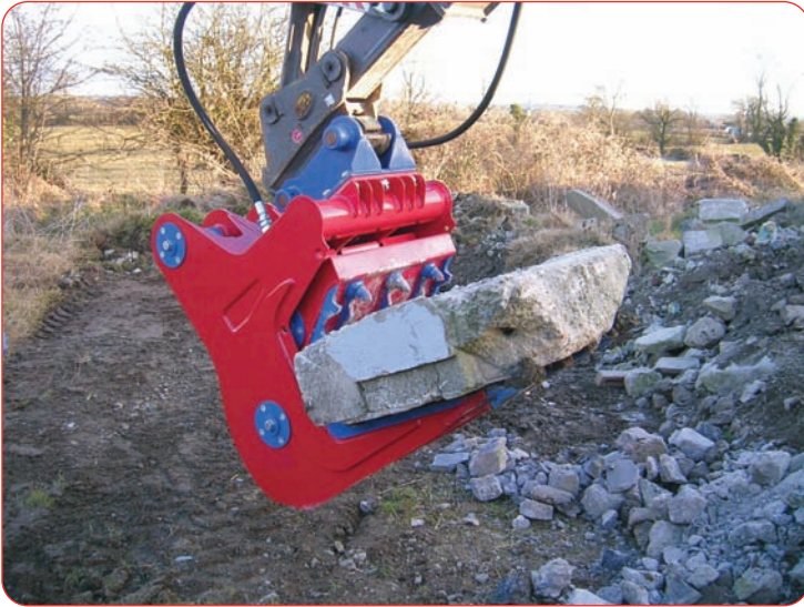
Easily crushes the larger rubble slabs.
